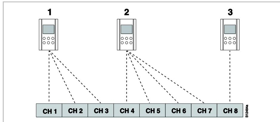
Fig. 65: Radio channel group with equal priority
