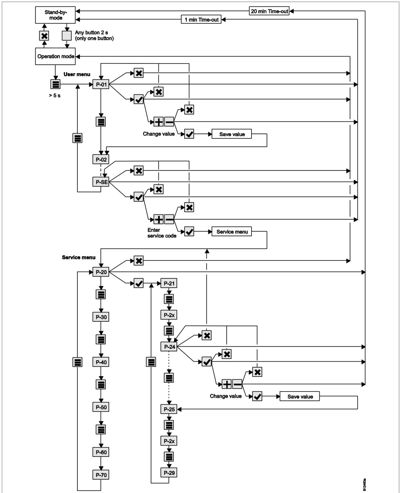
Fig. 64: Menu structure parameter settings for user and service level
