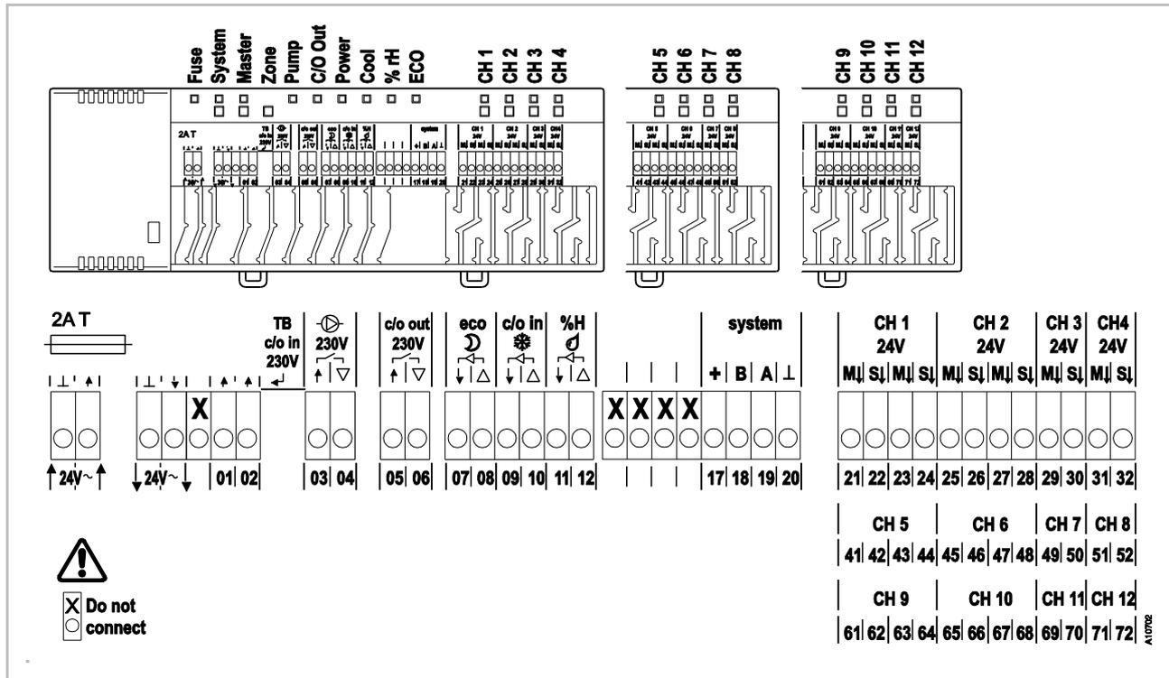
Fig. 24: Connection diagram, wireless connection modul 24 V version
