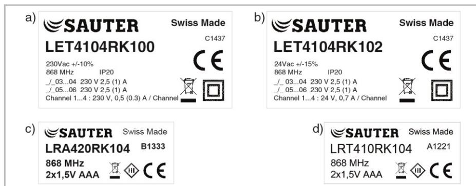
Fig. 1: Name plate a) wireless connection module 230 V b) wireless connection module 24 V, c) wireless room thermostat, d) Room thermostat with radio transmission, 24 V
