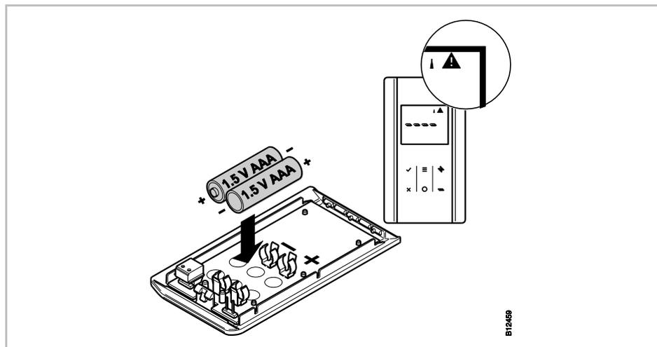
Fig. 14: Insert batteries
