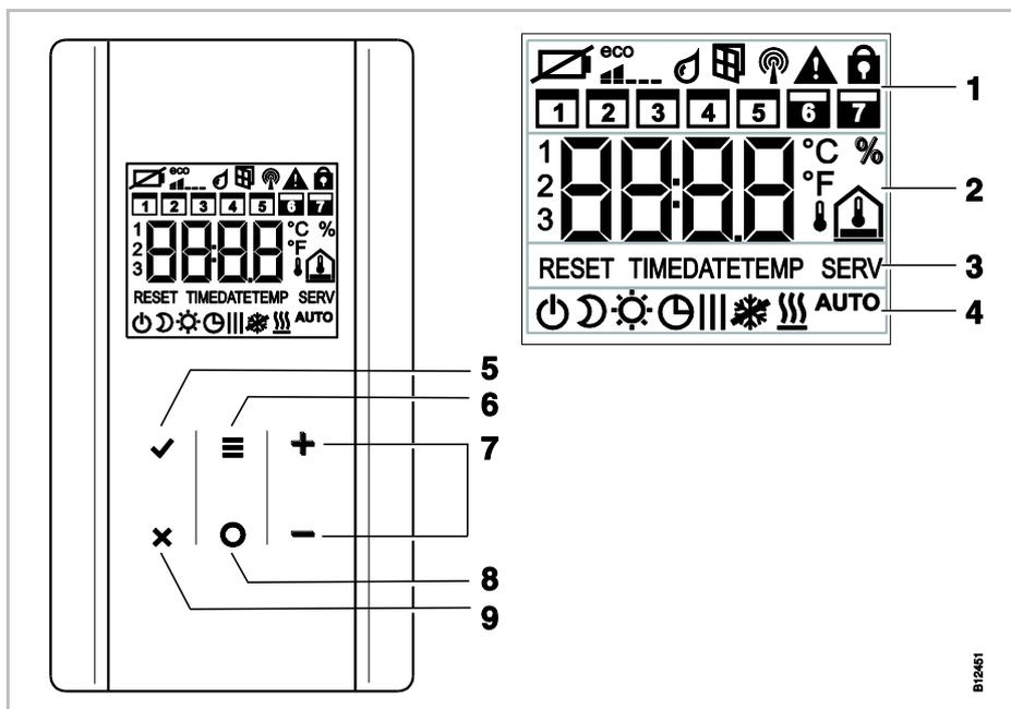
Fig. 5: Overview display and sensor buttons wireless room thermostat
