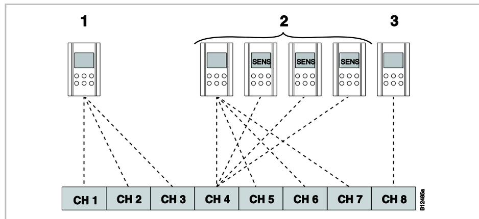
Fig. 66: Radio channel groups with equal priority and average temperature building
