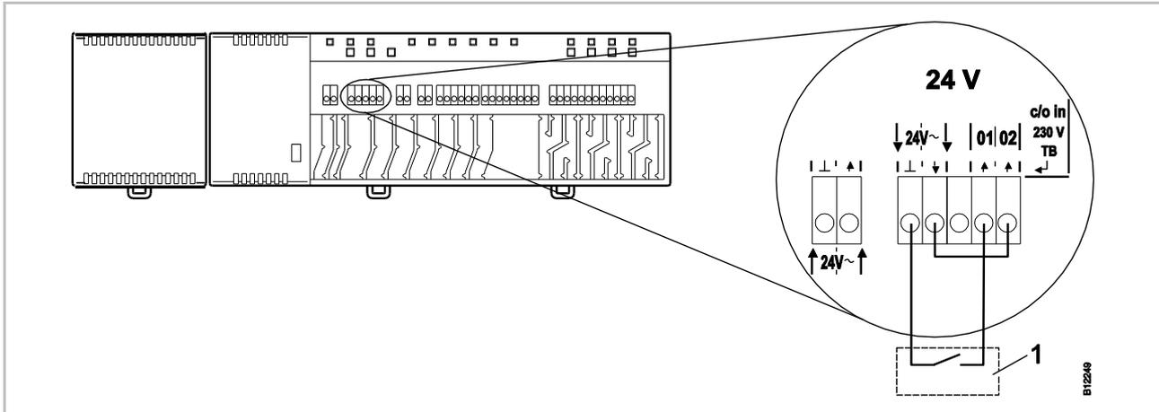
Fig. 29: TB-input, control with 24 V voltage from wireless connection module
