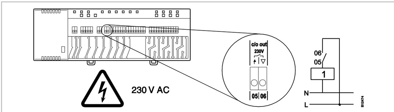
Fig. 44: C/O- or burner or ventilation control output, 230 V
