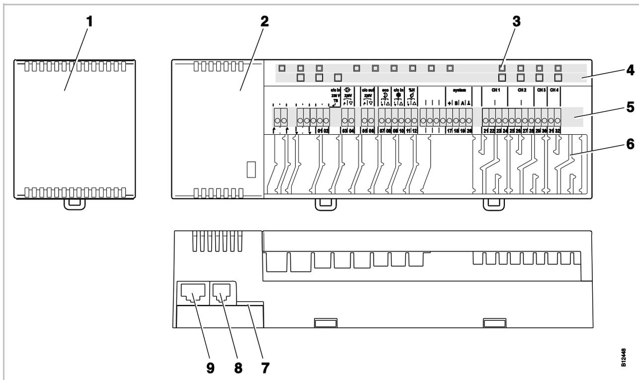
Fig. 2: Design wireless connection module, 4-channel version shown.
