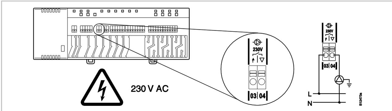
Fig. 43: Connect pump, 230 V
