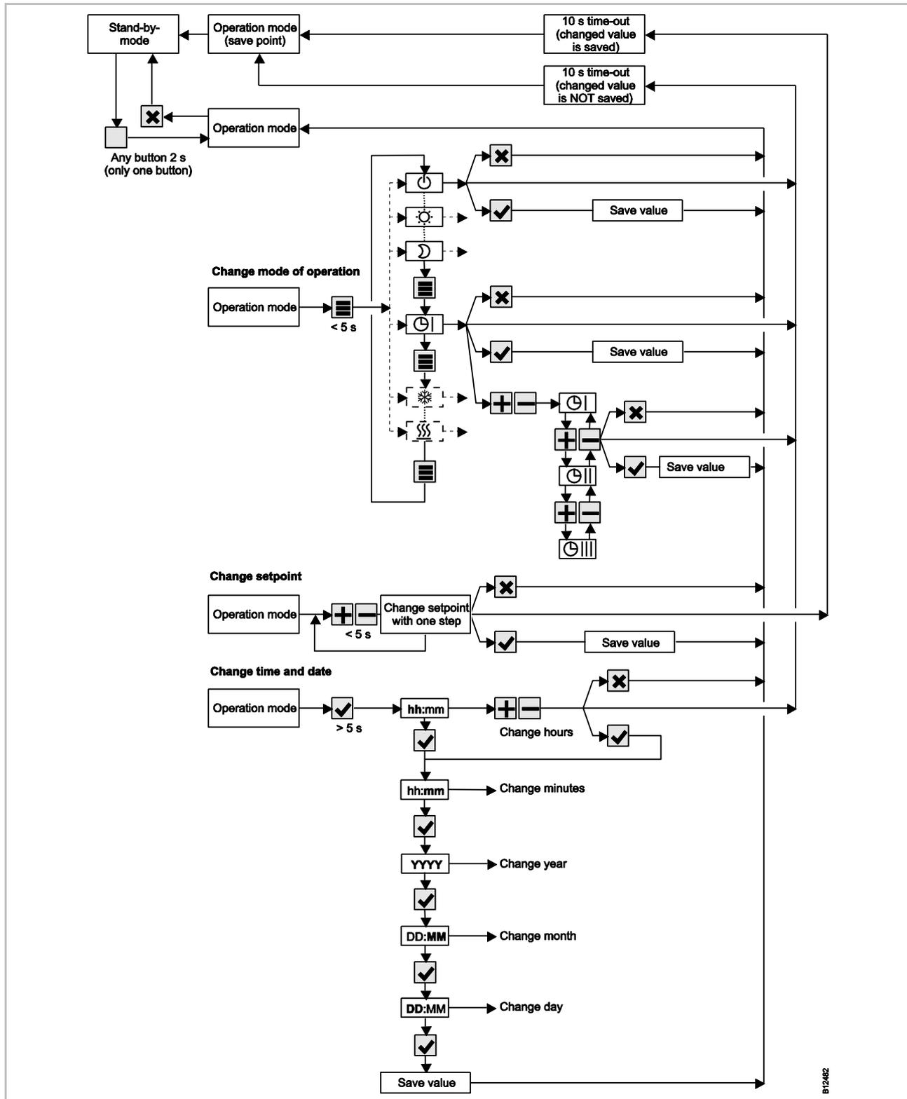
Fig. 63: Menu structure operation
