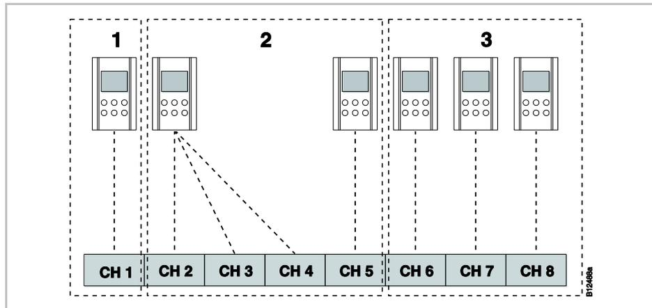
Fig. 69: Wireless room thermostat as "Master" for changing mode of operation
