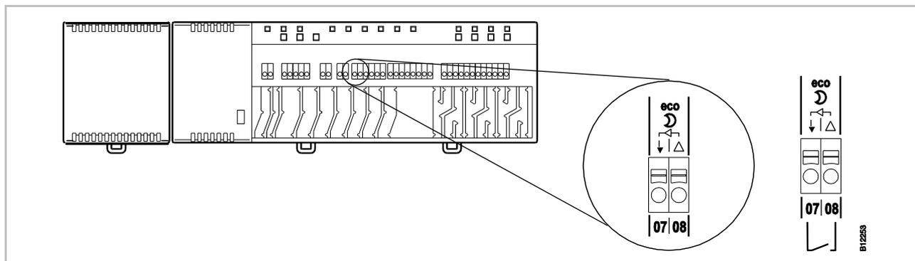
Fig. 33: Eco-input, contact recognition
