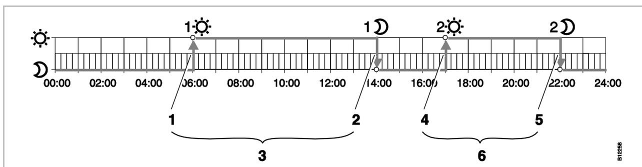
Fig. 50: Explanation "switched-on period" and "switching point"
