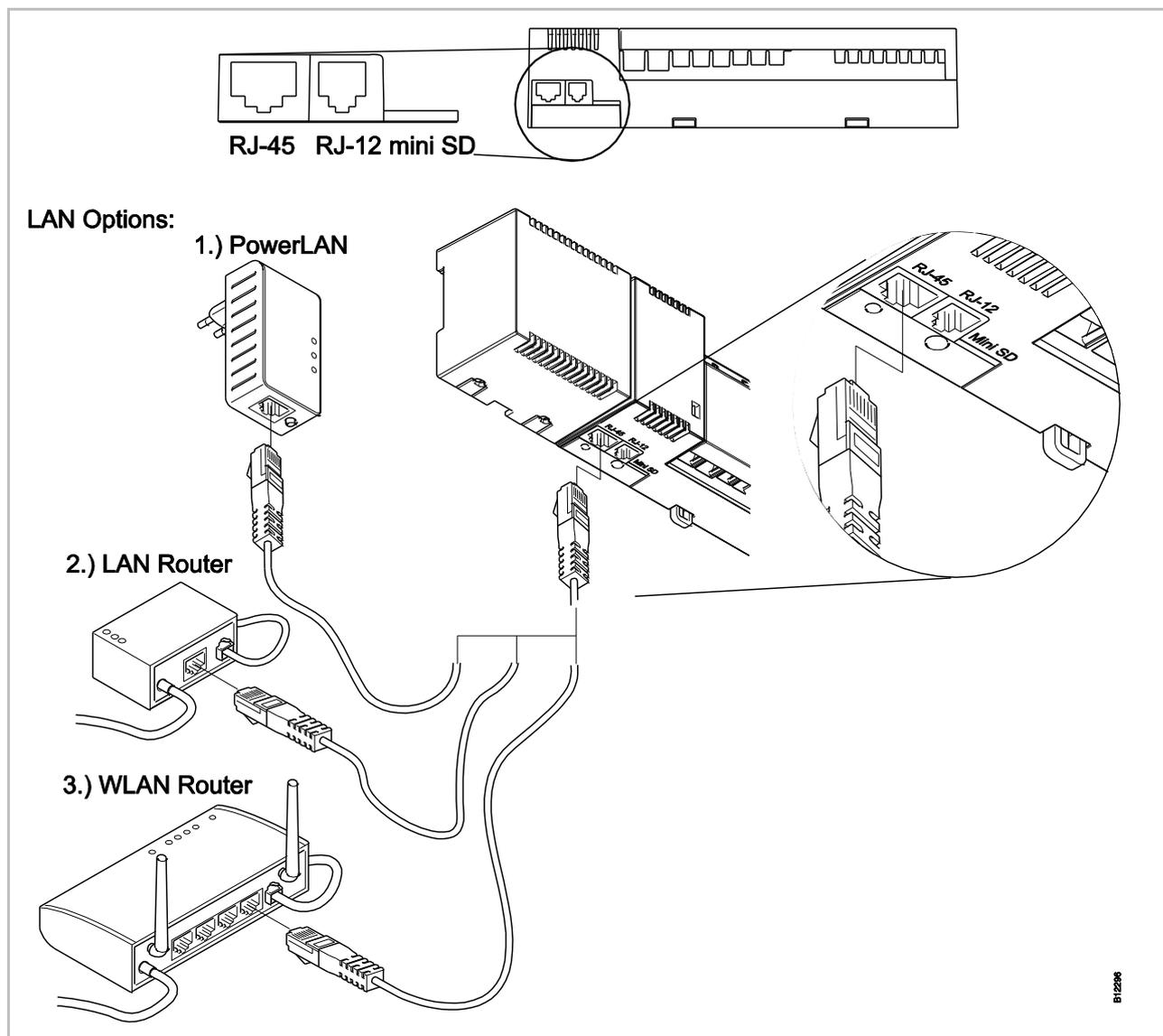
Fig. 49: LAN connection, here shown in the 24 V version with transformer
