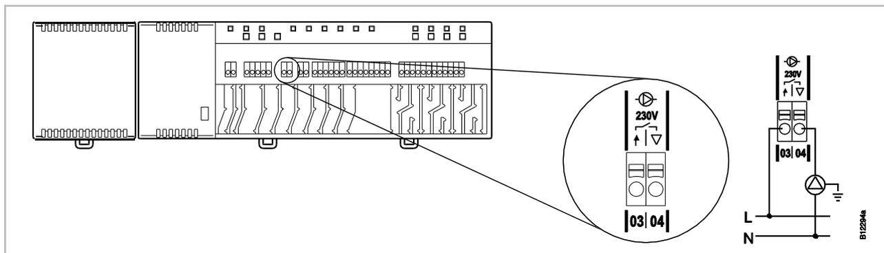
Fig. 31: Connect pump, 230 V
