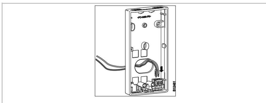
Fig. 16: Connect temperature sensor or window contact
