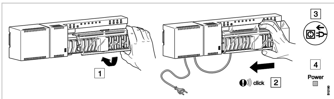
Fig. 36: Install cover and connect power supply
