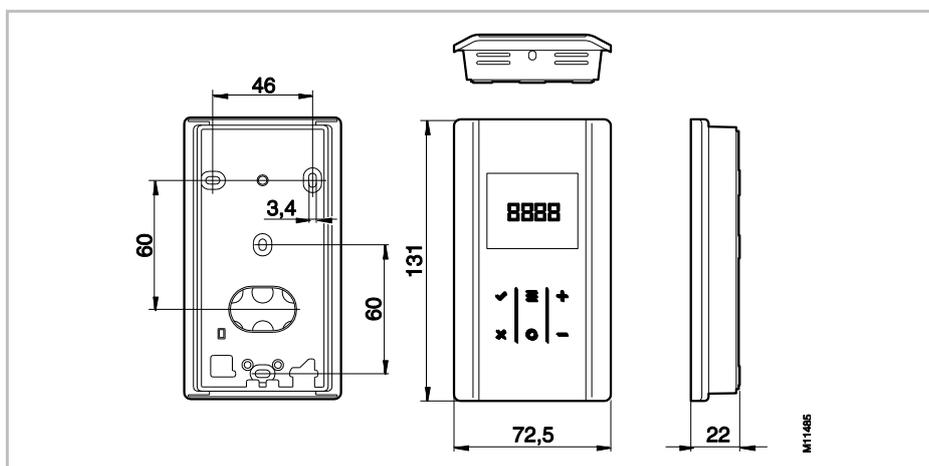
Fig. 60: Dimensions wireless room thermostat with display (all dimensions in mm)
