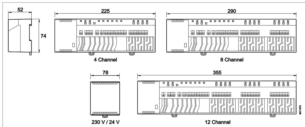
Fig. 59: Dimensions wireless connection module 24 V version and 230 V version and transformer for wireless connection module 230 V (all dimensions in mm)
