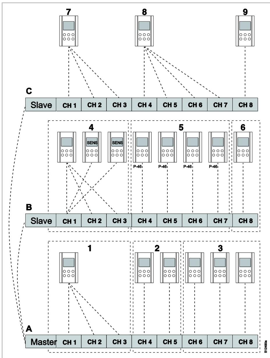
Fig. 71: Example with three wireless connection modules
