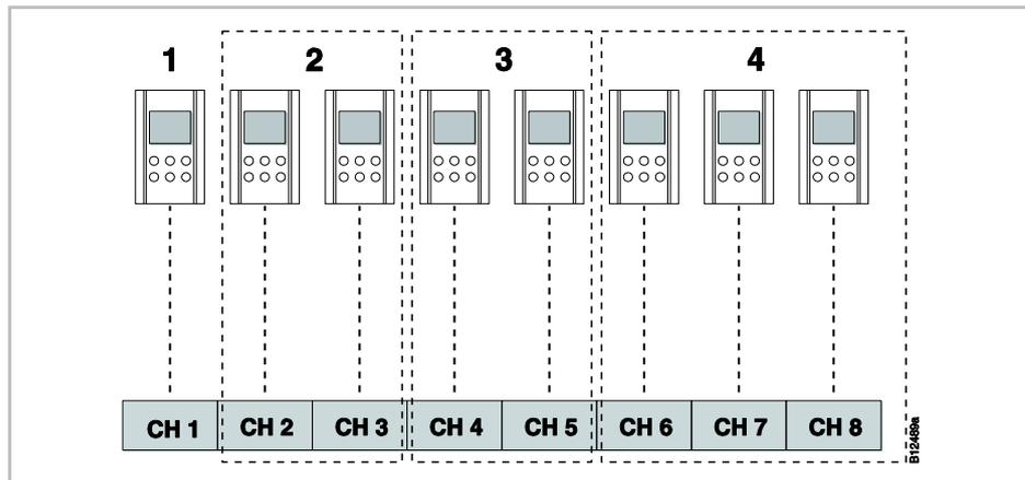
Fig. 70: Wireless room thermostat as "Master" for mode of operation
