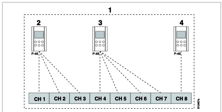
Fig. 68: Setpoint sharing for all wireless room thermostat within one zone
