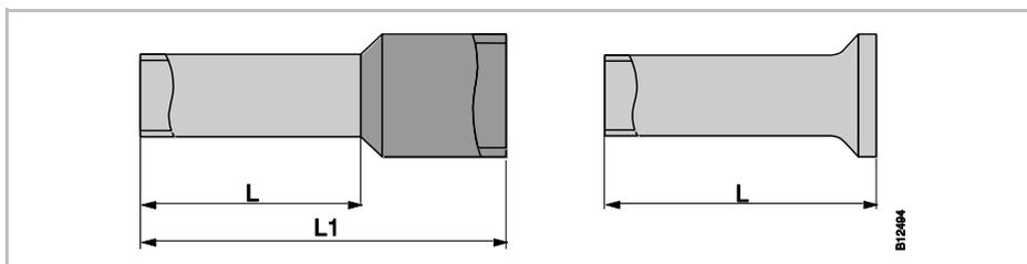
Fig. 22: Left: Wire-end ferrules with plastic collar
