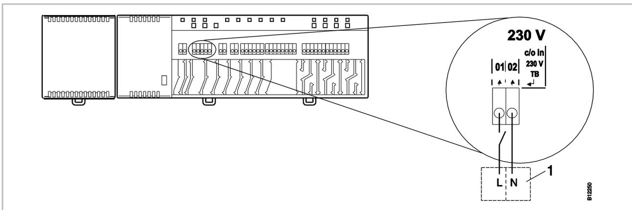
Fig. 30: TB-input, TB-input, control with 230 V
