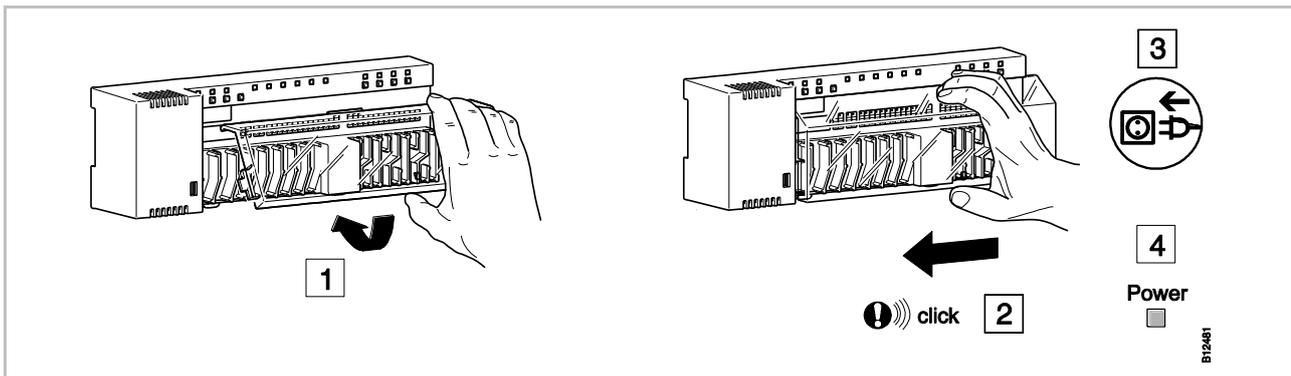
Fig. 48: Install cover and connect power supply
