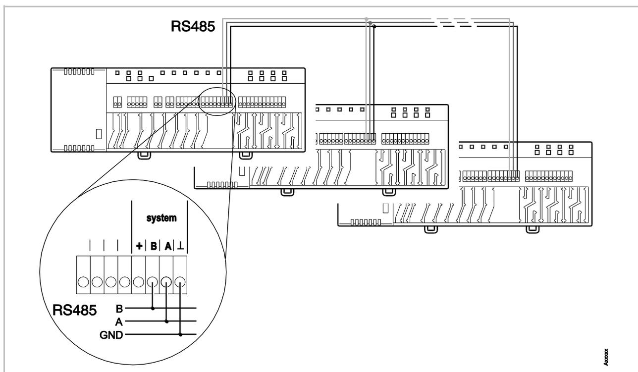
Fig. 56: Wiring bus system according to RS485 specification
