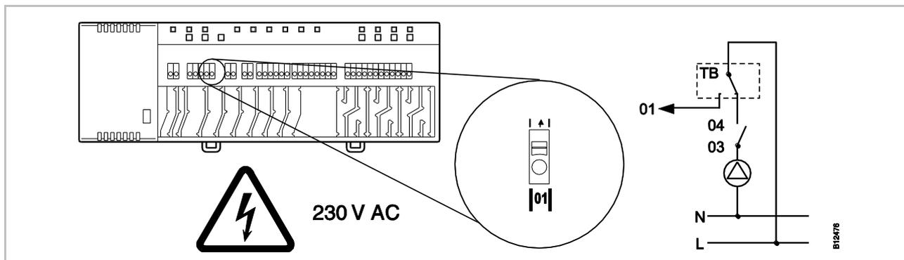
Fig. 41: TB- input for temperature monitoring
