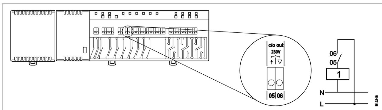
Fig. 32: C/O- or burner or ventilation control output, 230 V
