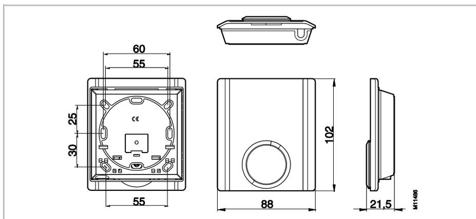
Fig. 62: Dimensions wireless room thermostat without display (all dimensions in mm)
