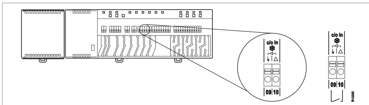
Fig. 34: C/O-input, contact recognition
