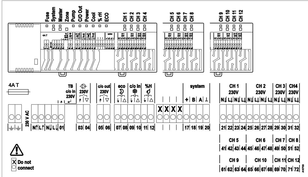
Fig. 37: Connection diagram, wireless connection module 230 V version
