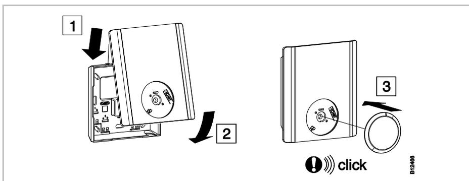
Fig. 21: Closing wireless room thermostat
