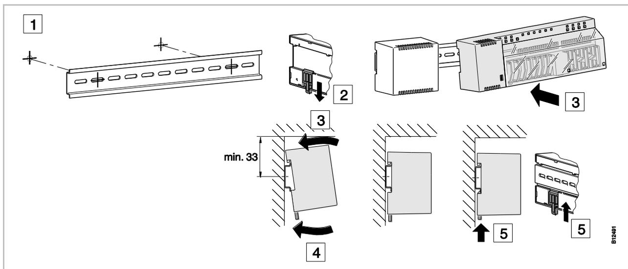
Fig. 8: Mounting wireless connection module, here shown in the 24 V version with transformer
