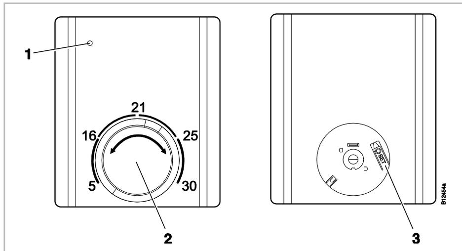
Fig. 7: Overview operating elements wireless room thermostat
