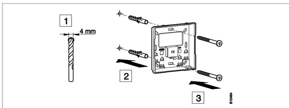
Fig. 19: Mount lower part of the wireless room thermostat
