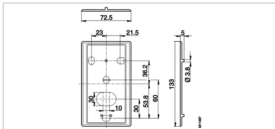
Fig. 61: Dimensions cover plate (all dimensions in mm)
