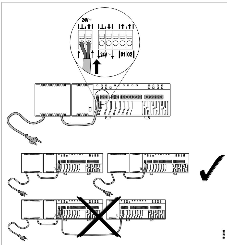
Fig. 27: Connect transformer
