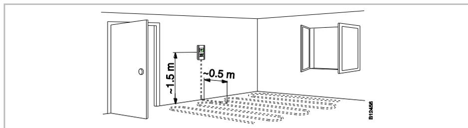
Fig. 11: Installation floor temperature sensor
