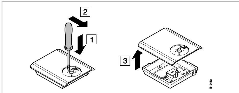
Fig. 18: Opening the wireless room thermostat
