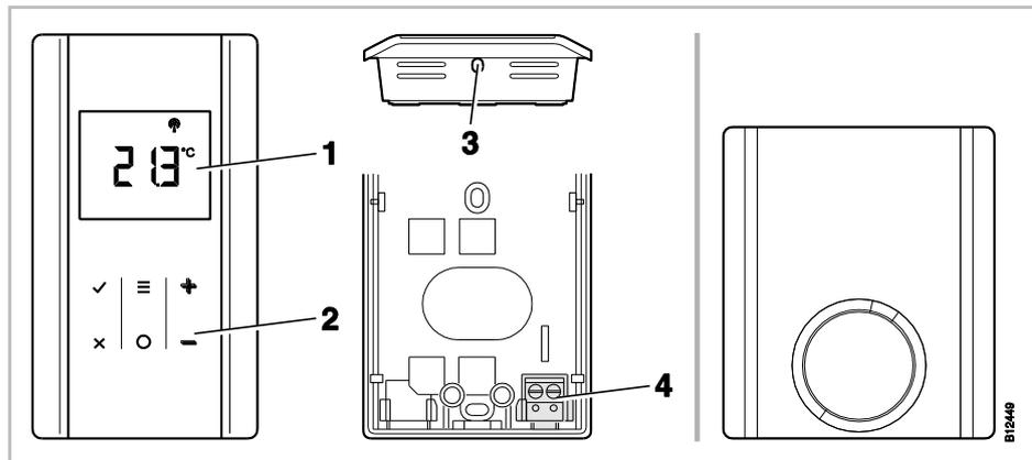
Fig. 3: Design wireless room thermostat, on the left with display, on the right without display
