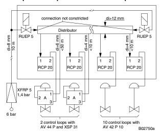
Typical air throughput  $\dot{V}_{max}$  at the distributor (see section 4.2)
