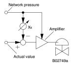
This effect becomes particularly serious if several devices of this type are connected to the same supply-air line or a poorly supplied manifold. In these cases, the positive feedback is transferred to all devices, pressure breaks down in the entire installation and the system may finally end up in a state of continuous oscillation.
