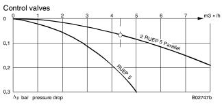
In order to estimate the total pressure drop, the air throughput rate  $\mathring{\mathbf{V}}_{\text{max.}}$  is determined according to 4.2) and the relevant  $\Delta p$ -values of the corresponding load curves are added up:
