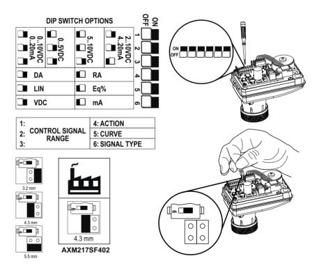
**DIP switches 1, 2, 3 and 6** DIP switches 1, 2 and 3 are used to set the control signal. The voltage (VDC) or current (mA) is set with DIP switch 6.
