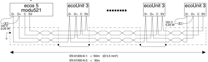
For industrial applications, the entire bus length may be max. 30 m to fulfil the criteria for interference resistance as per EN-61000-6-2. For residential, business and commercial applications with requirements as per EN61000-6-1, the entire bus length may be up to 100 m.
